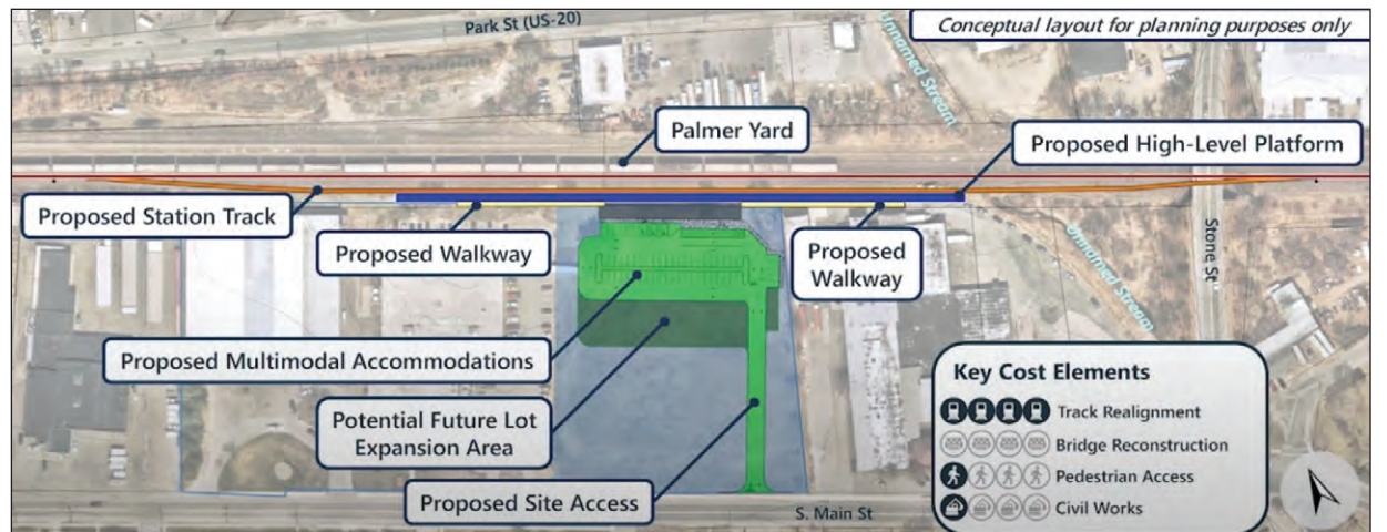
A draft diagram of how the proposed train station will fit into the selected site on South Main Street.
